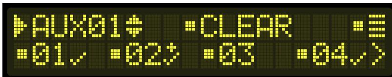
The LINK screen allows the user to edit the Link Table for the PRLC rack. The number of AUXIN channels in the Link Table is based on the number of PRLCs x 4.
